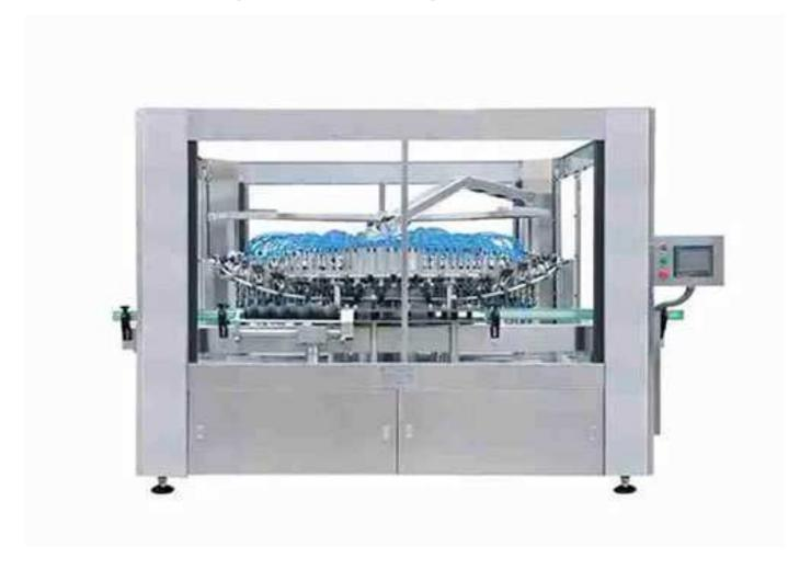
This bottle washing machine is mainly used for washing plastic bottles and glass bottles. The main production process consists of a flexible robot to grab the bottles, flip them, wash them, control them, and then flip and reset them. It is also equipped with a high-pressure pump for continuous tracking and washing, which realizes fully automatic washing.
