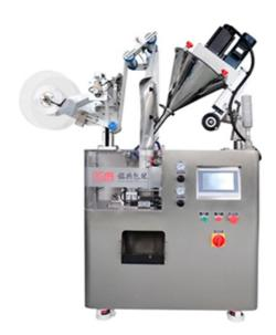
This machine adopts automatic following, tracking, positioning and so on; it does not require too much pre-parameter setting and adjustment during use, thus realizing the functions of one-click startup and one person operating multiple machines. This drip coffee bag packing machine has features like automatic measurement, inner and outer bag forming, and date printing, enhancing product safety.
