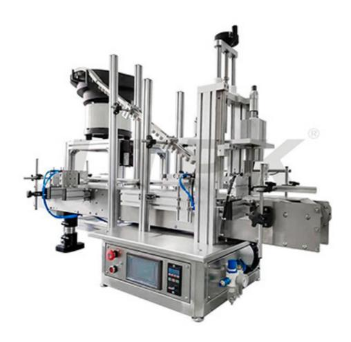
With a cap vibratory bowl, the machine can automatically sort and feed the caps. There is a rubber head for anchoring the cap. It applies 4 spinning heads to screw the cap, which makes it multipurpose. Also, it can be assembled with a filling machine and a labeling machine to form an automated production line.
