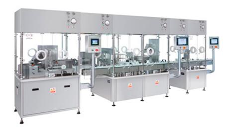
Eye drops production processors design compliances with cGMP/Pic/s of the sterile liquid product guideline. In order to meet this standard, the entire processors are built without any pneumatic accessories to prevent particles polluting production area.
