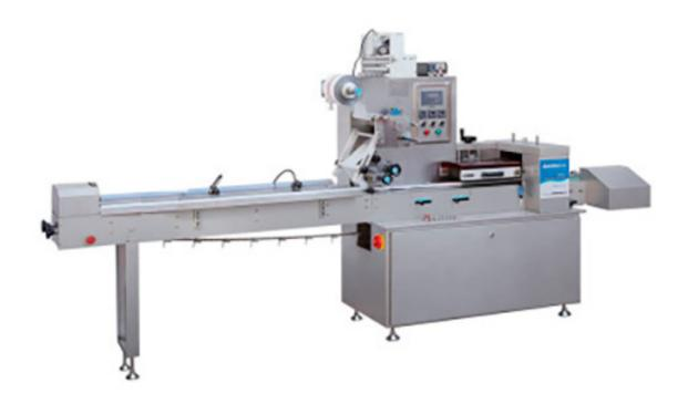
Automatic Flow pack machine or pillow packing machine is a rotary type packaging machine, that wrap many types of commodities including blister sheets, facial paper, soaps, biscuits, candies, chewing gum and instant noodles, and other rectangular, square, round or irregularly shaped products.
