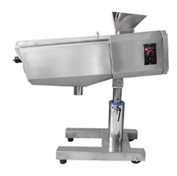
This is an automatic continues working tablet deduster, can be used with various types of press machine, which is main auxiliary equipment for the press. Which main function is removal powdery from the tablets. Connected with the vacuum cleaner and sucked out from the powder port. The machine is made of stainless steel, easy maintenance, corrosion resistant.
