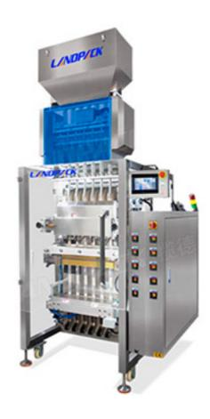
It is used for automatic filling of various granules into stick bags, such as sugar, salt, coffee, seed, sesame, desiccant, health products Industry and so on.
