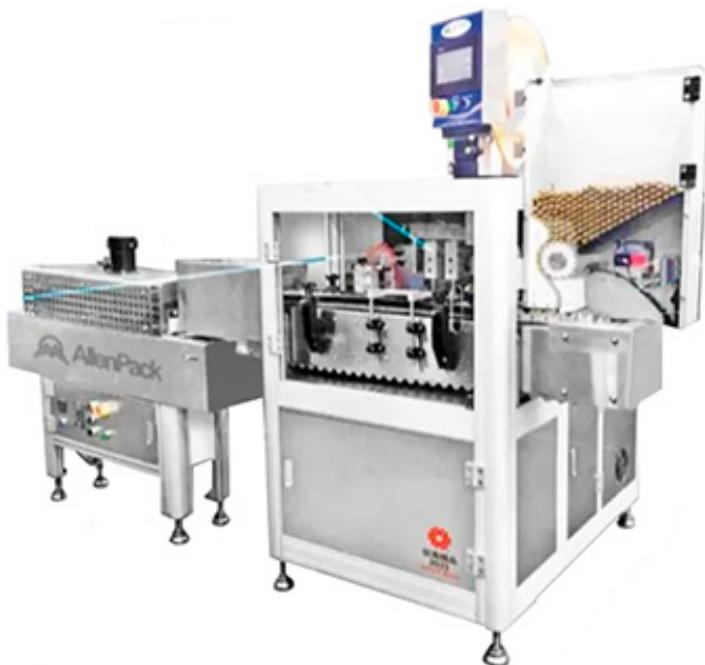
The automatic shrink sleeving machine from Allen Pack can easily be integrated with your company's existing packaging lines or we can also provide a complete system which would include the applicator, conveyor, and heat tunnel. It's suitable for all bottles with various width range and label position application.
