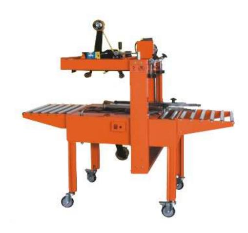
Carton sealers are case equipment that seals the top or bottom of a case with tape or glue. Typically, the minor corrugated flaps are kicked and plowed closed as the cases are transferred. As the cases enter the compression section, the major flaps of the carton are closed and a hotmelt adhesive is applied.
