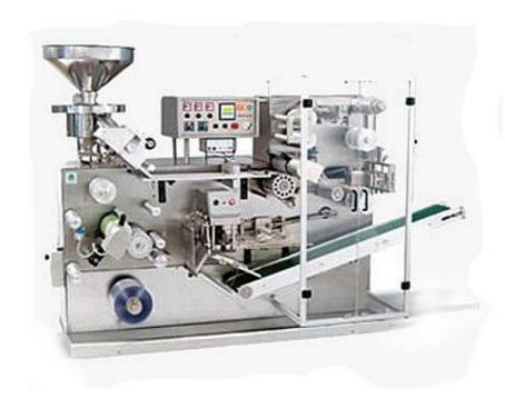
The machine is thermo forming standard basic machine PVC ALU
