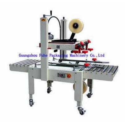
Carton sealer machine is mainly use in packaging case, not only working alone but also work with production line. It is widely use in household appliances, spinning, food, general merchandise, medicine, chemical industry, etc. Top and side drive carton sealer machine is general suitable for tall case.
