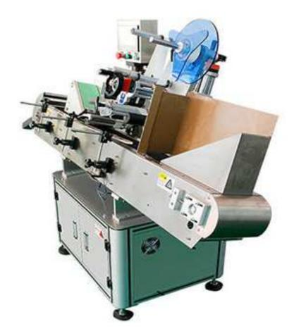
HL-T-402 Suitable for the unstable circular cylindrical objects, semi circle labeling, horizontal transmission, horizontal labeling way, increasing stability, improving the labeling efficiency.
