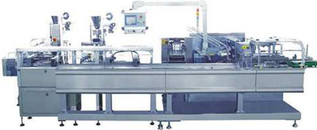
Suitable for single or multi-bag packing of granules, powders and liquids in bags.
