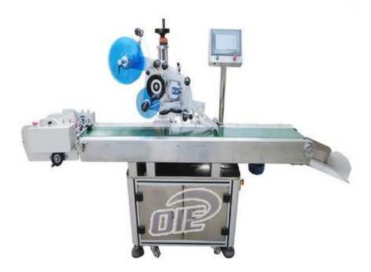
OL-812 automatic self-adhesive flat labeling machine well designed for labeling all kinds of cards, and labeling protective film on plastic sheet.
