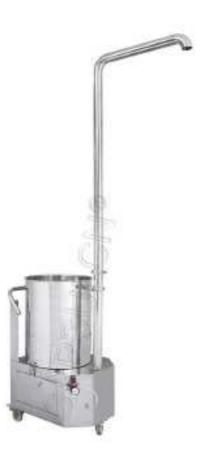
The JNJ Empty Capsule Conveyor is a simple and efficient method for the gentle and repeatable transfer of empty capsules into the capsule filling machine.
