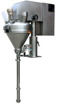
Specialized design for granulates or powder, widely apply in food industry, products such as milk powder, glucose powder, milled coffee, rice powder, milky tea powder, milled spices, dried cream, flour mixes, instant drinks etc. Metering screw driven by servo motor, particularly suitable for requests high accuracy, high speed and more stability occasions. Whole machine are made of stainless steel, could be washed directly by water, meets the food industry requirements.
