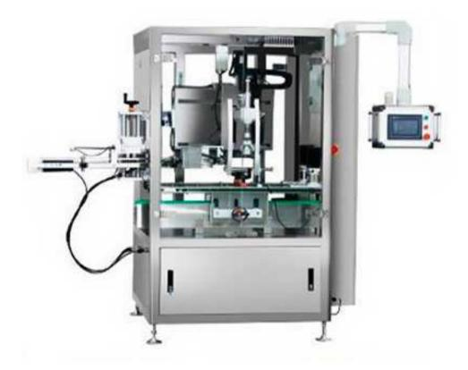
This capping machine adopts advanced servo motor control technology. Uses 6 sets of servo motors to control a single capping head. In the process of capping, capping head automatically locates the position of bottle neck, and moves with the bottle after grasping the cap to screw the cap.
