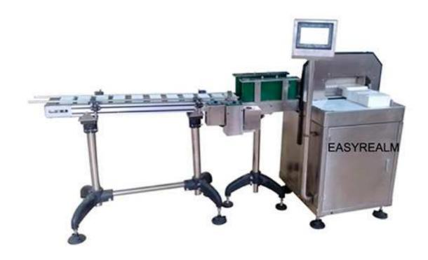
This automatic banding machine, with the box/carton collating & stacking system, is for automatically bundling pharma boxes by film strip.
