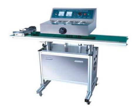
The LGYF-2000-BX continuous induction sealer utilizes electromagnetic induction principle to produce instant high heat to melt aluminum foil. Then it adheres to the bung hole, reaching the aim of wet-proof, leakage-proof, mildew-proof and extending preservation time. Now it is widely used as sealing package machine in industries such as pharmaceuticals, pesticides, pesticides, lubricant and cosmetics etc.
