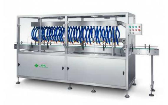
It is suitable for various kinds of irregular-shaped bottles and standard bottles. With such features as stable performance, good drying effect, no dust pollution caused by brush, simple operation, maintenance-free, low energy consumption and no wearing parts, it is currently the ideal drying equipment.
