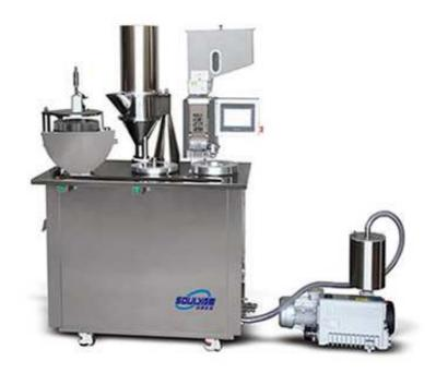
This model is an intermittent motion and hole plate type filling full automatic capsule filling equipment. It adopts an optimization design for meeting the characteristics of Chinese medicine and the requirement of GMP, it has the characteristics of compact mechanism, small volume, lower noise, precision filling dosage, multi-function, stably running, etc.
