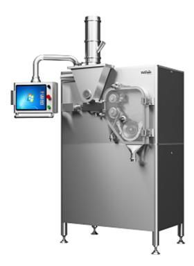
During granulation, the dispensed and mixed dry powder materials are fed into the upper hopper through the special feeder (pneumatic or mechanical) and conveyed to the pressure chamber through the spiral conveyor. The two high pressure extrusion wheels will press the materials into slices of high pressure density, which will be cut into small pieces by the cutting system and made into granules of desired sizes by the two-stage granule sizing system, so that the granulating process is completed.
