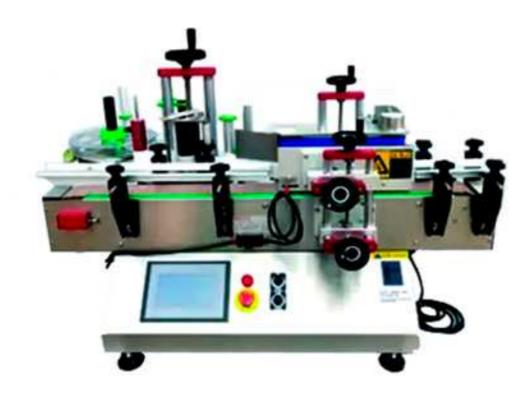
This machine is used to label the adhesive label on the round bottle. This labeling machine is suitable for PET bottle, plastic bottle, glass bottle and metal bottle. It is a small machine with low price which can put on desk.
