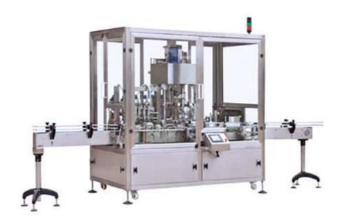
This production line is suitable for the filling production of small batch multi-gauge, liquidity or viscous materials. It only needs 2 operators to complete filling, capping, labeling and packing. The line structure is compact, small footprint, which will help the workshop planning and adjustment.
