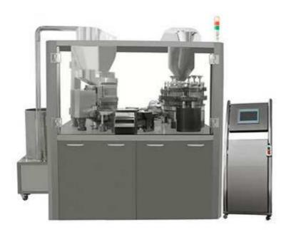
GTI-C Series Automatic Capsule Filling machine adopts PLC and HMI control system and international famous brands electronic components, such as Mitsubishi, Simens, Schneider, and Omron etc. The machine is widely used in pharmaceutical industry, health-care products etc.
