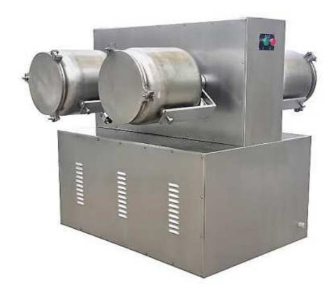
Single-chamber ball mill FQ120 is a horizontal rotating device. It uses 2 methods of grinding: the dry grinding and wet grinding. This mill comprises elements for loading and unloading materials, parts and rotary elements of the transmission. Currently, the mill is used to grind very fine grinding of materials in the pharmaceutical, chemical and food industries, as well as in scientific research, etc. In addition, one-ball mill to mix the materials capable of at least two substances.
