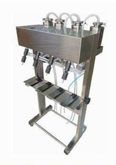
Perfume filling machine is used for filling floral water, perfume and other water-based materials. The machine adopts negative pressure and liquid surface type filling. It includes two kinds of specification such as four-head and six-head. Explosion-proof type products can be provided according to user requirements.
