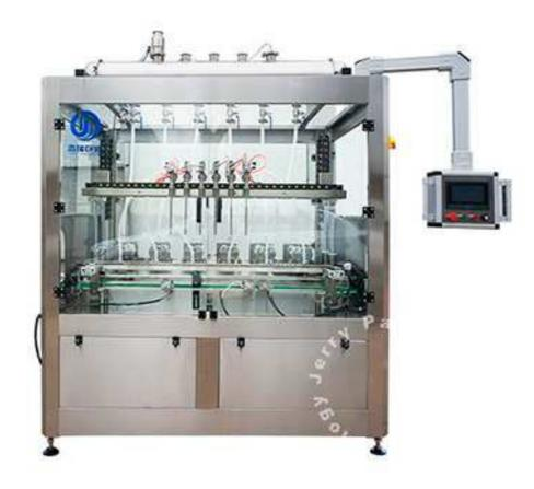
JLF series filling machine adopts high-precision rotor lobe pump to measure the liquid capacity. Each pump is driven by a servo motor, with a wide filling range and high filling accuracy.
