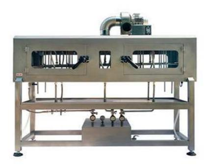
Steam wrapping tunnel is used for shrinking sleeve labels to label kinds of bottles: different and irregular round bottles, square bottles, flat bottles and women-shaped bottles. By shrinking PVC or PET sleeve labels to seal bottles caps /necks, cover bottles body even shrink wrap bottle bottom.
