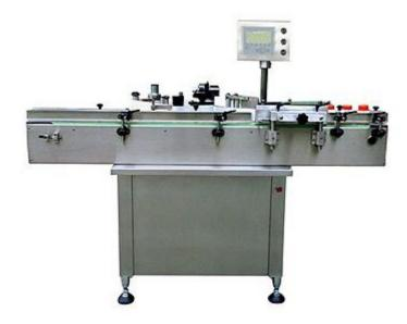
The sticky labeler applies sticky roller to label on small round bottles. In the process of vertical bottle feeding, label is torn off consecutively from the labeling roll and stuck on the fixed position of the bottle body. It is a modern machine integrating mechanism and electricity with good and reliable working property.
