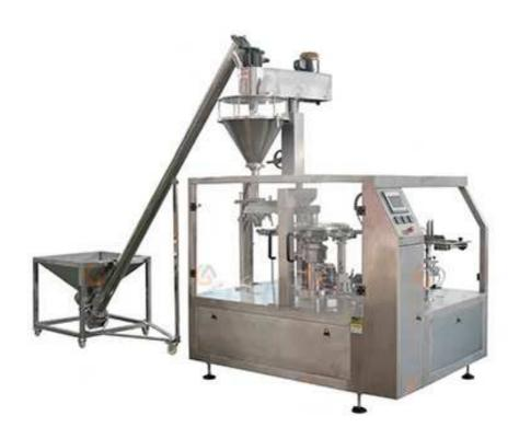
Fully Automatic Spice Powder Packing Machine suit for packaging flour, milk powder, corn starch, soy flour, glucose powder, ice cream powder, pepper powder, fish food powder, curry powder, cocoa powder, coffee powder, bean powder, washing powder, alkaline powder, organic fertilizer, etc.
