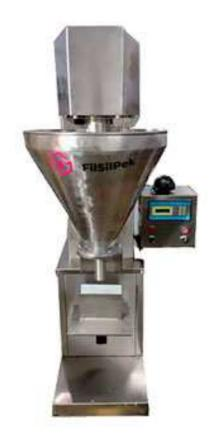
Semi automatic Auger type Powder filling machine is precision built on sturdy welded MS frame completely enclosed in stainless steel sheet and doors are provided to facilitate the servicing of machine. The unit is made compact, versatile and enclosed in stainless steel elegantly matt finish body.
