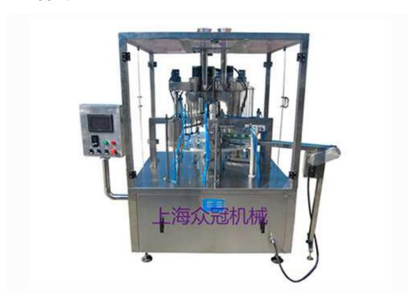
BHZ (rotation type) Cup filling and sealing machine is widely used in various kinds of plastic cup for liquid filling and sealing. It can automatically finish the process of filling, sealing, cutting, printing the code, sterilizing in ultraviolet radiation and falling cup etc. In addition, it can be customized that according to your special requirements.
