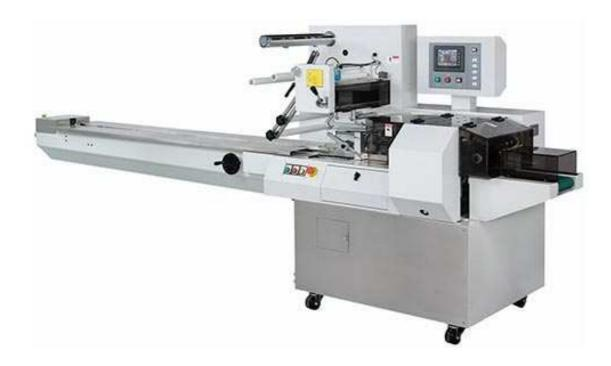
3-axis servo flow wrapper. Seal data, product data can be recorded. Adjusting is simple and fast.
