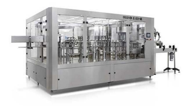
The CGF series Wash-filling-capping 3-in-1 Machinery is used to mineral water bottling process, purified water, flavored water and other non-carbonated beverage as well. The CGF Wash-filling-capping 3-in-1 machine can finish all the process from empty bottle rinsing, filling and sealing, it can reduce the materials and Outsiders touch time, improve the sanitary conditions, production capacity and high cost effective.
