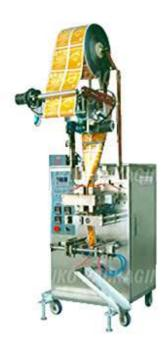
The MK-213 is a Fully pneumatic Vertical (VFFS) form fill and seal packaging machine designed to package viscous liquids and paste products. This Fully automatic Vertical packaging machine uses volumetric pneumatic paste pump filler system to produce center sealed, 3 side sealed and 4 side sealed pouches / bags.
