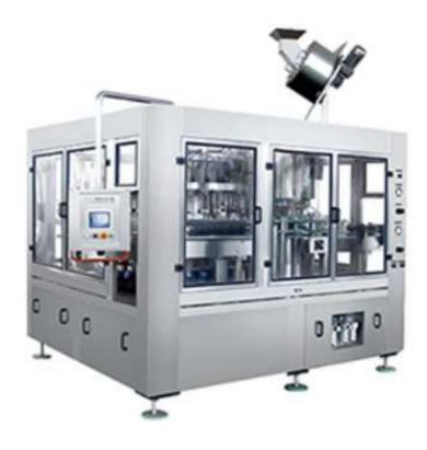
The series of filling machine for carbon dioxide-free wine, beverages, spices and other liquid quantitative filling glass bottles.
