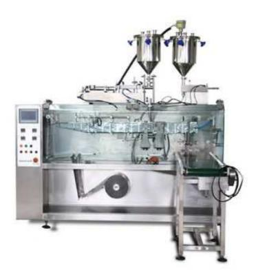
This machine is designed with new vision of innovation, for producing the best product. It's working with 30 gr, and in optimum conditions it can reach 100 packs per minute. Also when it's producing our first goal was supply safe working for workers, that's why we add a safety part on it. For all of the electronic and pneumatic parts used world-known brands. And also this machine has half cut unit.
