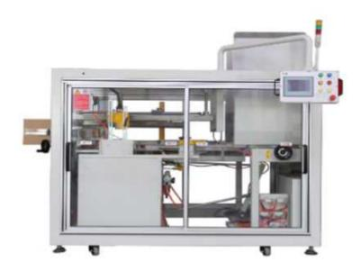
This machine is designed for the second packing of the flexible bags packing, which need to put into the carton case.
