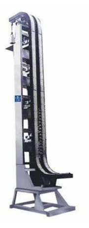
Vertical conveyor for USCP450 bottles designed for vertical transport of containers: bottles, bottles, cans and other containers for infusion solutions. It can be used in conjunction with other transport equipment.
