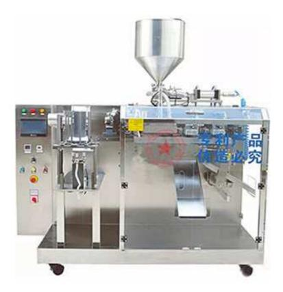
This mini bottle shape pouch packing machine does premade stand up pouch picking up, filling, sealing and shape cutting fully automatically.
