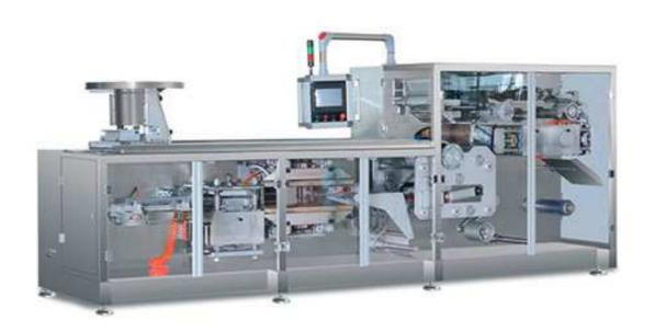
DPH330E Blister packing machine is our company new develop high speed machine which combines the advantage of plate-type and rotary-type machine. With the international high level technology concept, full servo motor, bus control system, modular design, high feeding capacity, intelligent and low noise. Easy operation and mold exchange. Meet GMP quality standard. It is widely used in medicine, health care products, medical devices and electronic components blister packing.
