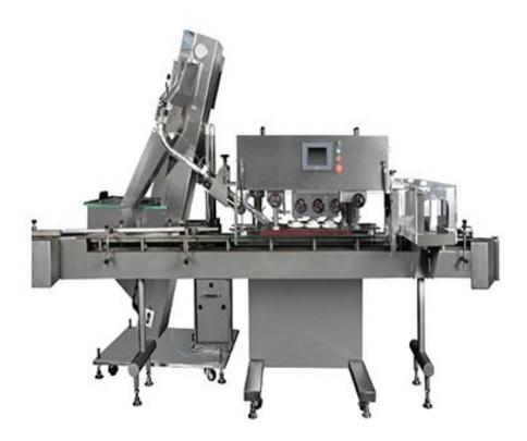
This is one of the perfect capping machines with sound quality. The machines supply a capping solution to various shapes of plastic bottles. The latest and developed technologies adapted to this equipment ensure the speed and accurate work stably.
