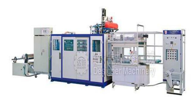
Mostly the ZKD70-200 cup thermoforming machine with stacker is able to make different kinds of cup, bowl, container, plate and lid by changing the molds. The products could be in various plastic materials such as PP, PS, PET, PVC and Bio degradable material.
