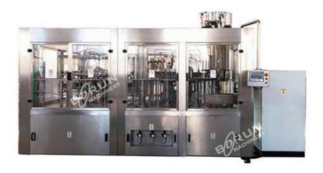
This Full Automatic Soft Drinks Filling Capping Machine For Glass Bottle is mainly used for carbonated beverage filling capping. The machine is 3 in 1 monoblack composed of washing, filling, capping in one unit. The rinsing head adopts overturning device, and filling system is gravity filling type, it's more stable and reliable.
