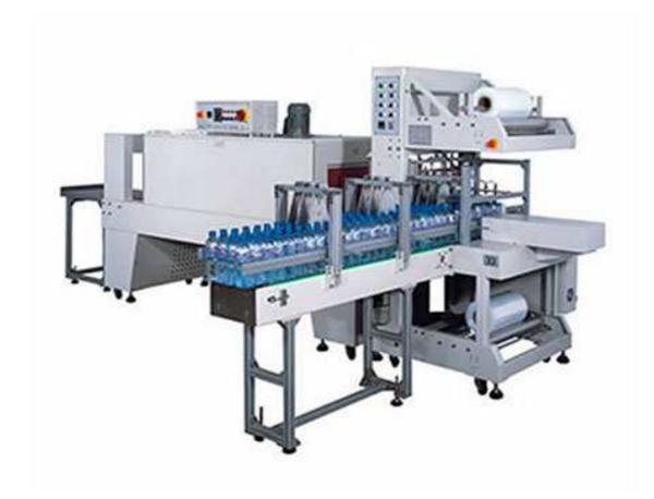
BZS-800 is suitable for wrapping products such as pop-cans, bottles, etc, with bottom-tray or without bottom-tray, working with BZS-400 or other PE shrink tunnels.
