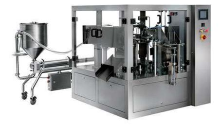
This automatic packaging machine unit is specialized in liquid and paste such as juice, ketchup, béchamel, capsicum paste, liquid soap and edible oil etc. This machine includes the rotary packing machine can liquid & paste filler.
