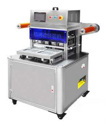
GT640 Fresh meat food fruit tray gas flushing sealing machine also called Automatic modified atmosphere tray sealing machine.
