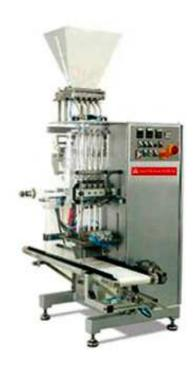
PLC control unit, servo motor controlled film transport, connection apparatus and hoses for aspirator group. Metallic grey colored and surfaces of the machine that are in contact with the product made stainless
