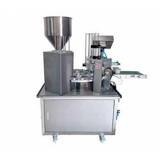
This machine is a full-automatic filling and sealing machine, through PLC controller and various pneumatic electronic accessories to achieve automatic cup drop UV sterilization (optional), automatic filling, automatic sealing, automatic coding (optional), automatic capping. The finished product is automatically sent to the assembly line to realize mass production
